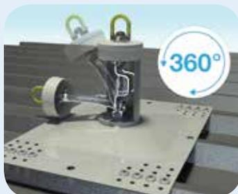
**360° protection :** In the event of a fall, the Söll Fusion® Roof Anchor Post collapses in the direction of the force, the built-in, energy-absorbing component activates and the base remains securely attached to the roof surface.
